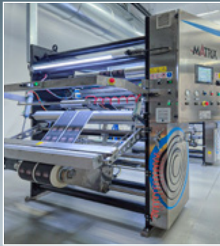
Rewinders and "doctor machine", up to 500 mt/min
